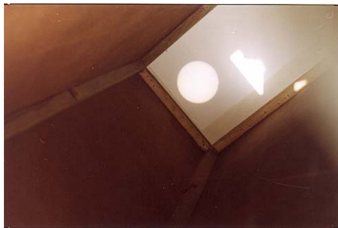
Projected image of the Sun inside a hardboard box, using binoculars
